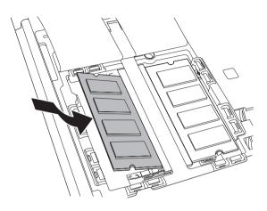
Figure 8-13 Installing a memory module
